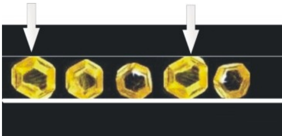
Fig. 1: Illustrating Limited Points of Contact Ungraded Diamond Powder Resulting in Scratch Formation
